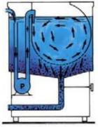
TURBOVER exclusive washing system consists of a washing drum, perforated on the sides and on the bottom, and an outer basin, where the pump intake is placed near the main water inlet.
